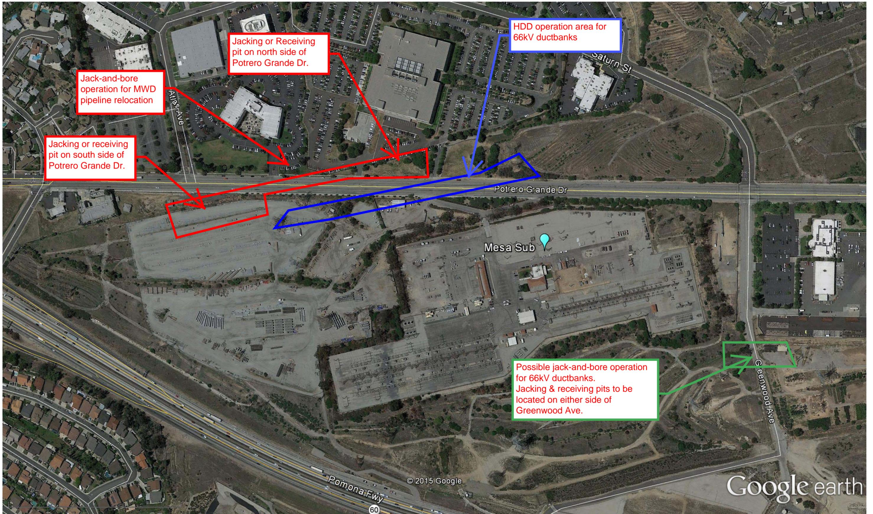
Jack-and-bore operation for MWD pipeline relocation
